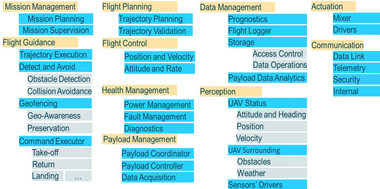
Figure 23: Overall blocks of a drone system
