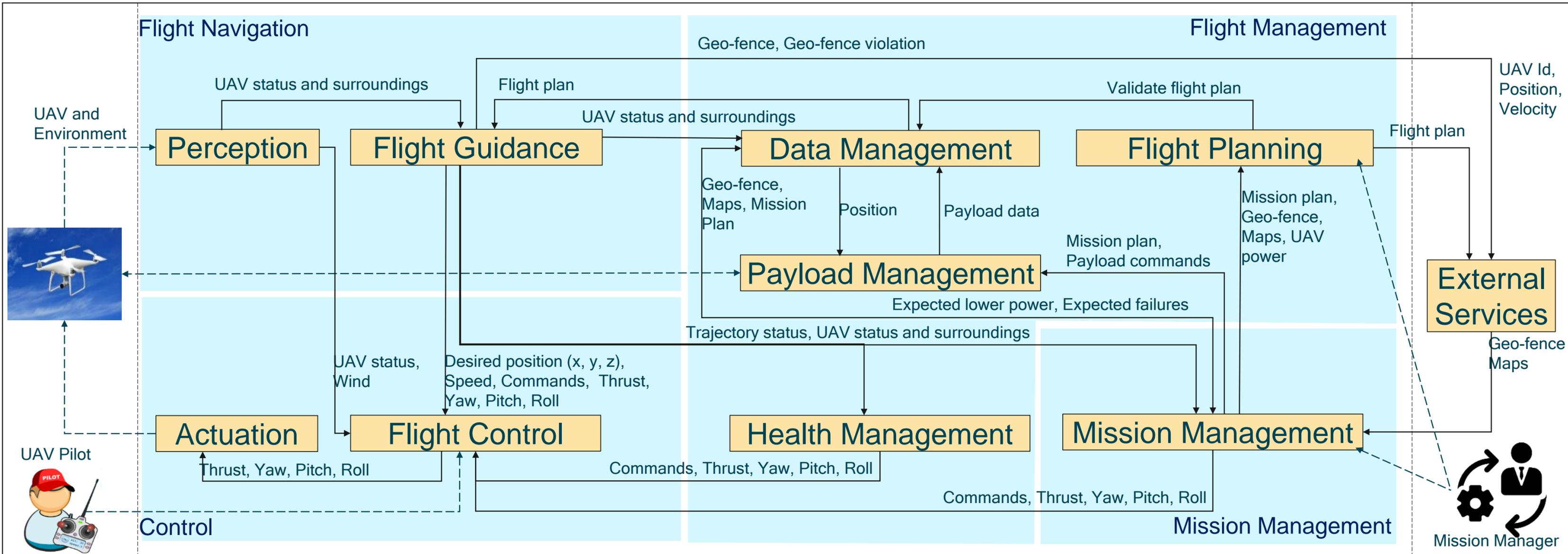
\*UAV status: Actual Position, Attitude, Velocity, Power Level, Engine(s) status, ...
